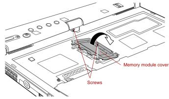
Figure 3-10 Removing the memory module cover
